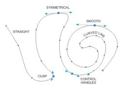
Figure 6: Different types of nodes
